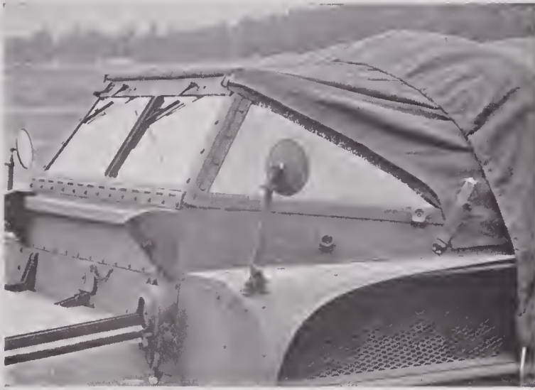
FIGURE 31. Final production windshield developed to withstand surf impact.
